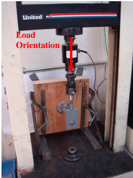
Figure 2a. Shear Perpendicular to Rafter
